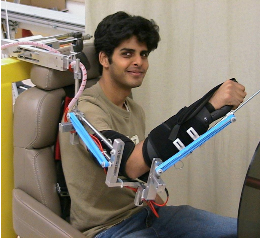
Therapy/Training-Wilmington Robotic Exoskeleton (Sanchez et al. 2004)
